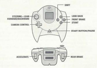
Never touch the Analog Thumb Pad or Triggers L/R while turning the Sega Dreamcast power ON. Doing so may disrupt the controller initialization procedure and result in malfunction.
